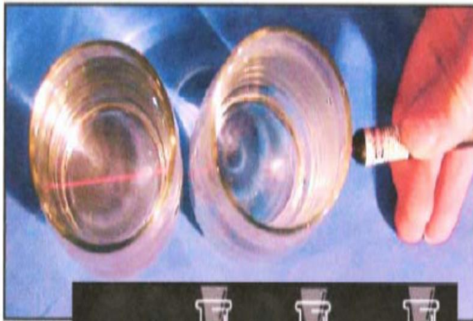
Tyndall Effect: Laser Pointer traveling through a solution (right) and through a colloidal suspension (left).
